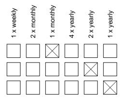
Check foundation, foundation anchoring and whole construction for corrosion, repair or replace if necessary.
