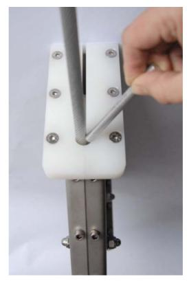
The 8 mm finger rod shall not pass through the opening!
