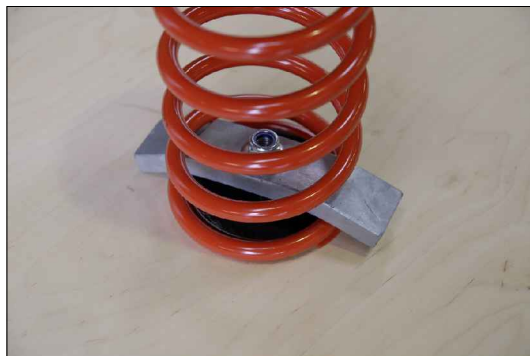
3 x screw connection totter platform on compression spring/holder consisting of: mushroom head screw M12x80-DIN603-zinc-plated; safety nut M12-DIN985-zinc-plated;
